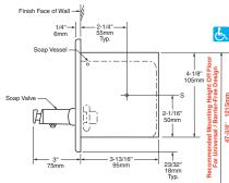
Rough Wall Opening 8-3/8" (210mm) wide 4-3/8" (110mm) high 3-7/8" (98mm) minimum recessed depth
