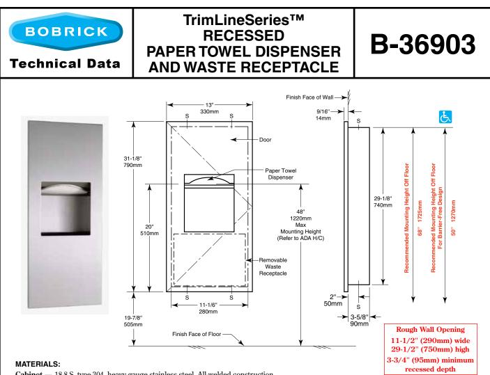
Cabinet — 18-8 S, type-304, heavy-gauge stainless steel. All-welded construction.
