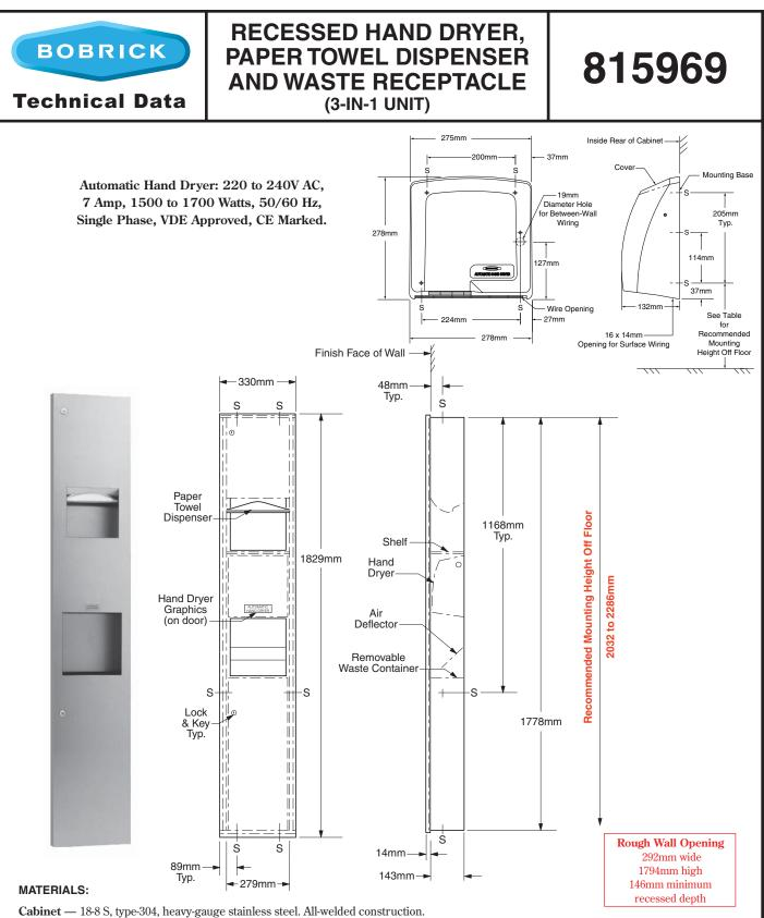
Door — 18-8 S, type-304, 1.2mm (18-gauge) stainless steel. 14mm 90° return for maximum rigidity. Secured to cabinet with a concealed, full-length stainless steel piano-hinge. Equipped with a stainless steel cable door-swing limiter and two tumbler locks keyed like other Bobrick washroom accessories.
