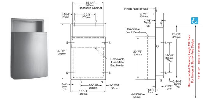
Rough Wall Opening 15-7/8" (405mm) wide 26-1/4" (665mm) high 4" (100mm) minimum recessed depth
